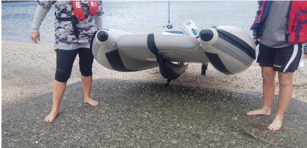
When inflated (250mbar / 3.6PSI), the Speed-Tube is attached to the rings of the bow fixation under the connecting floor and additionally fixed centrally to the lower transom bar, on the left and right side of the transom plate, using the two tension straps supplied.
